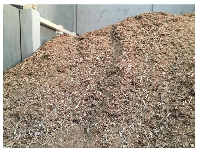
...fresh hogged fuel with wood sizes up to 350 mm and 45 to 55% moisture content and bark to fuel New Zealand's most advanced energy plant
