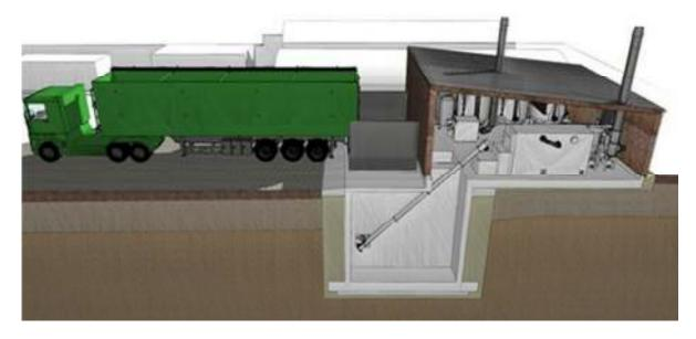
The design of the fuel delivery and storage is influenced by the types of truck options available. For a walking floor or tip truck, the above design would work well and there are numerous other delivery and storage designs including:
